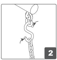
2. Use the Bender Tool to bend the S hook completly. All S-hooks must be bent fully closed.
