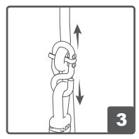
You will need to insert the loop of the long rope into the end of the "8" shaped hook, close the pin and pull snug. You can adjust the rope as needed to fit your swing set.
