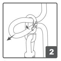
Create a loop in the long ended rope near the base of the seat and in the other hand take the "8" shaped hook.
