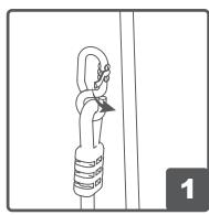
Open the pin on the 8" shaped hook.
